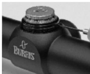
The click values can vary between scopes. The click value for your scope is noted inside the dust cover on either the windage or elevation knob.
