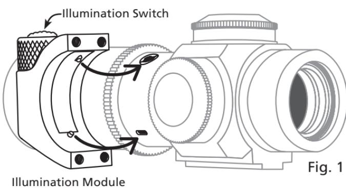
4. Align the other half of the module with the 4 screw holes and secure the screws (12-15 inch/lbs).
