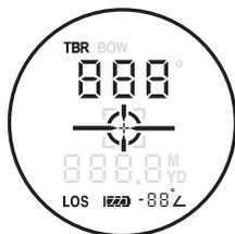
For rifle users, TBR mode is comprised of three functions: Hold, MOA, and BAS. One of these modes must be selected. To select the desired function, activate TBR, then proceed through the menu (by pressing the MODE button), past the BOW and Compass functions, until the appropriate TBR function is flashing; use the POWER button to activate the appropriate TBR function.
