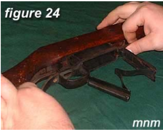
24) Replace magazine cover and install screws .
