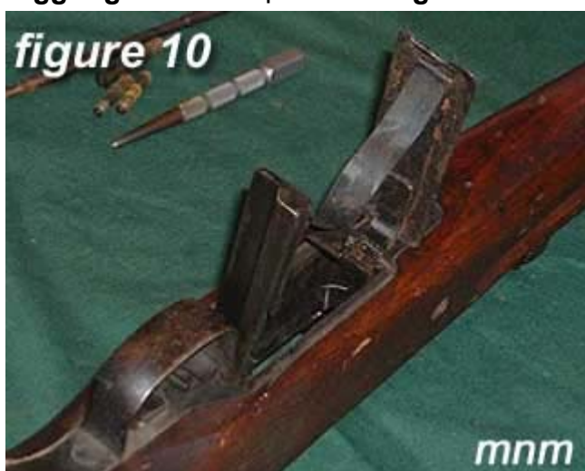
10) Figure 10 shows the magazine cover opened.
