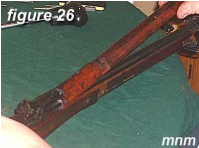
26) Place the handguard back onto rifle .
