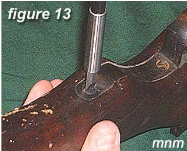
13) Remove the rear trigger guard screw .
