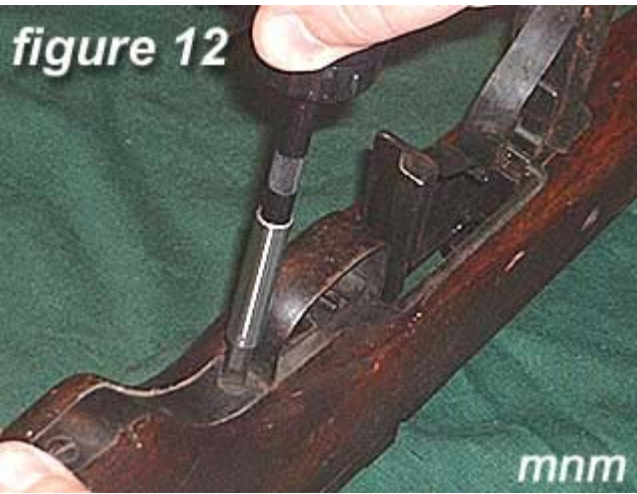
12) Remove the middle trigger guard screw .
