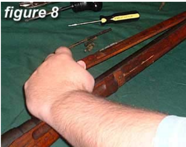
8) Remove the handguard and set aside.
