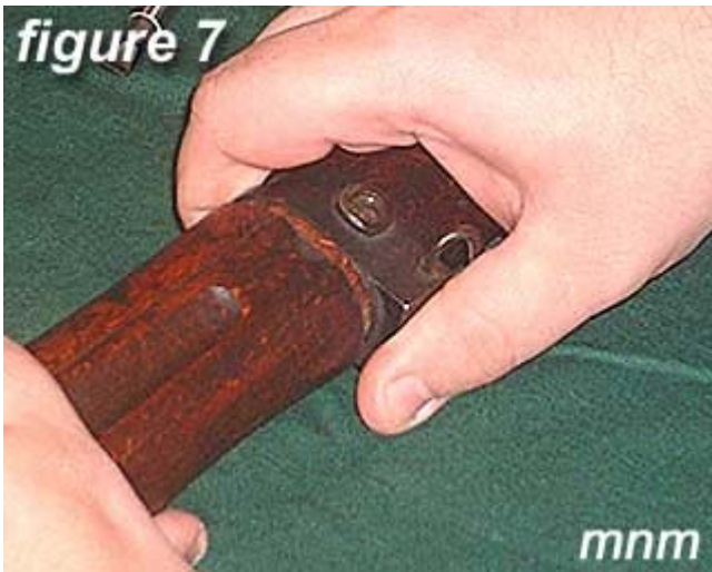
7) Slide the rear barrel band forward.
