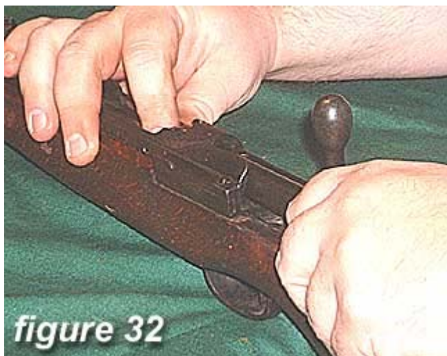
32) Slide bolt into receiver while pushing down on the magazine follower.
