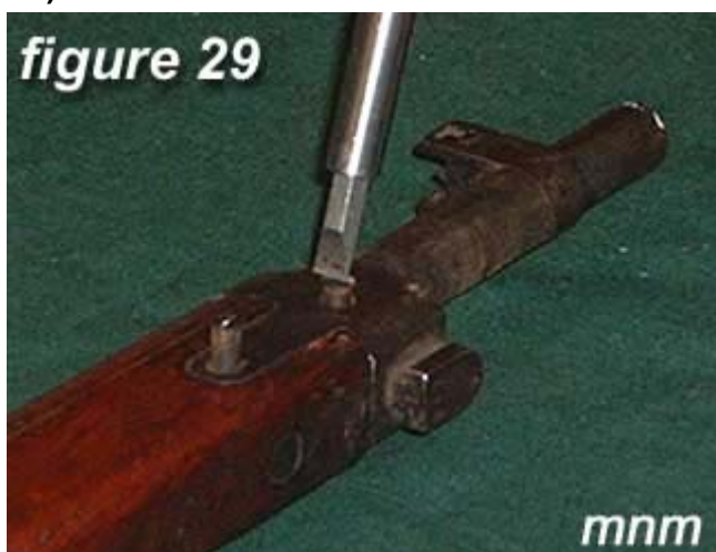
29) Replace forward barrel band screws and tighten.
