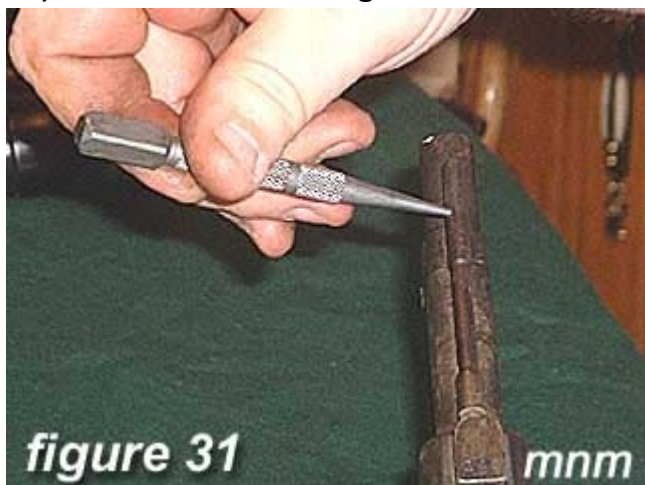
31) Use a small punch to insert in hole in front of stacking rod and rotate until tight.
