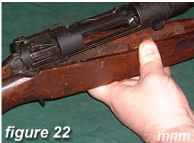
22) Place barrel and receiver assembly back into the rifle stock, resting on top of the receiver tang.
