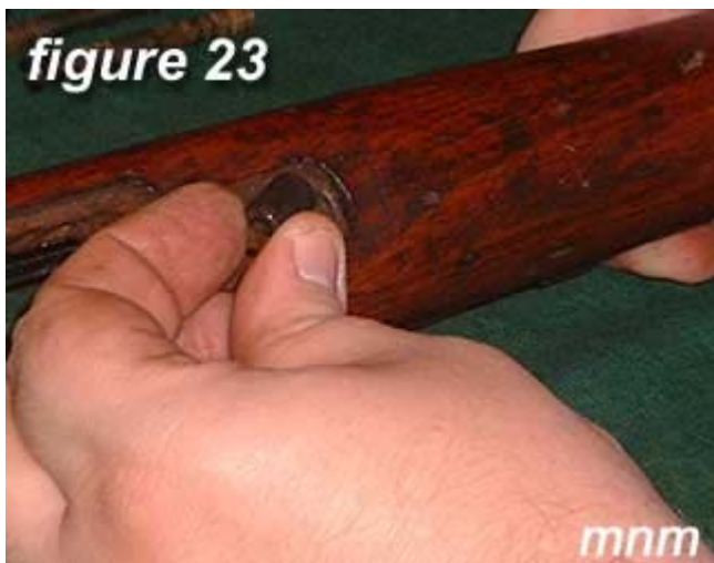
23) Place screw bushing back into front trigger/magazine assembly retaining hole before reinstalling trigger/magazine assembly.
