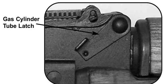
Rotate the gas cylinder tube locking latch upward to free the gas cylinder tube.
