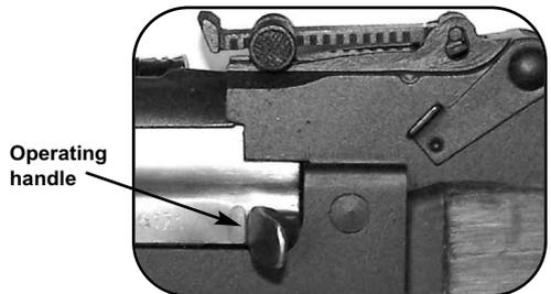
The operating handle is drawn to the rear to check the rifle's loaded/unloaded status.
